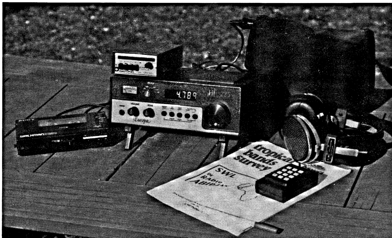
Figure 7. The author's portable DX listening station includes the HF-225E, Datong ANF, Sony Walkman Pro WMD6C cassette recorder and a 12VDC rechargeable battery pack.
