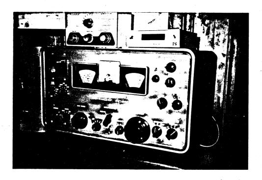
FIGURE 2. The author's HQ-180A with Q-multiplier and digital readout resting on top of the receiver. Note the non-stock oversized bandspread tuning knob.
