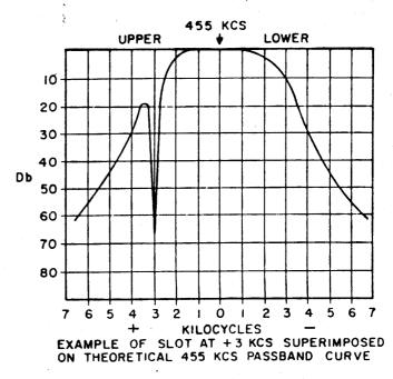
FIGURE 3. An example from the HQ-180A owner's manual showing the performance characteristics of the excellent notch, or slot, filter.
