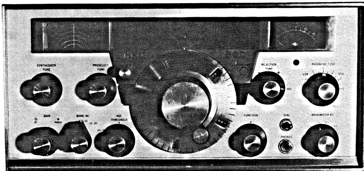
FIGURE 6. The HRO-500 was the last of the line that was built for ordinary mortals like you and me. When it was introduced in 1965, the receiver was truly state-of-the-art, using an advanced tuning scheme called crystal synthesis that made every frequency it tuned as stable as if it were crystal controlled. Crystal synthesis differs from the phase-locked loop arrangement common today in that frequencies are produced by heterodyning crystal oscillators against one another. It's a purely analogue technique that's inherently quieter than the digital schemes used today. This fine specimen belongs to David Clark.
