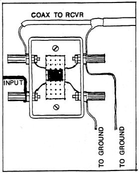
MICRO-CIRCUIT BASED IMPEDANCE TRANSFORMER
