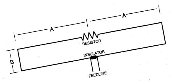
The T2FD has a characteristic 5 or 6 to 1 frequency ratio, which means that it works effectively from its low-end design frequency up to 5 or 6 times that frequency. For instance, the T2FD which I use is designed for optimum performance at 4.9 Mhz, but can operate up to the 25-29 Mhz range. In practice this antenna also works satisfactorily down to the 75 & 90 meter tropical bands, but not as well as a dipole or delta loop designed for 75 or 90 meters.
